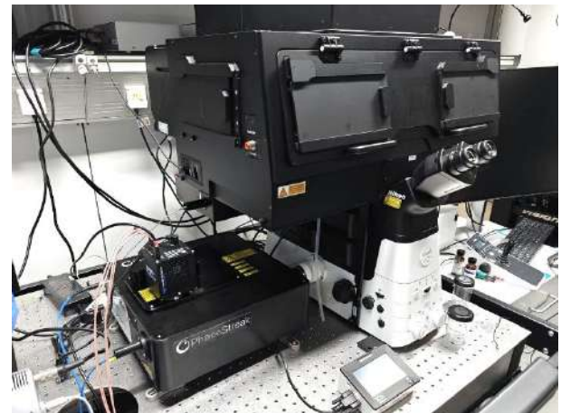
Fig. 1 A SENSOCELL+ platform integrated with PhaseStreak Confocal installed on a Ti2-E motorized microscope with incubation chamber at the Technical University of Dresden, Germany (Jan Brugués Lab)
