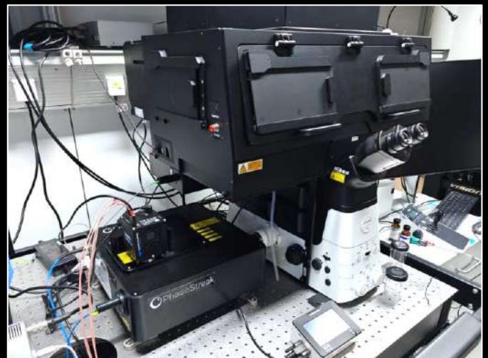
PhaseStreak integrated with SENSOCCELL+ optical tweezers on an inverted microscope at the Jan Brugués Lab, TU Dresden, Germany.
